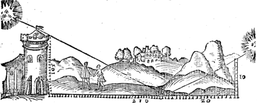
Fig. 4.17: Measuring a tower using the sun from Digges (1571, Sig.D1 v )
